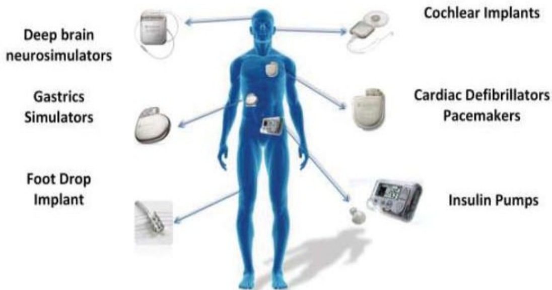
Figure 6: Smart biomedical measurement devices (implantable measurement devices)
