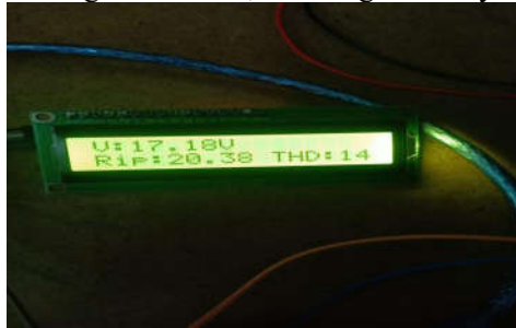
Fig 5.4.2 Output in THD Meter as observed With filter
