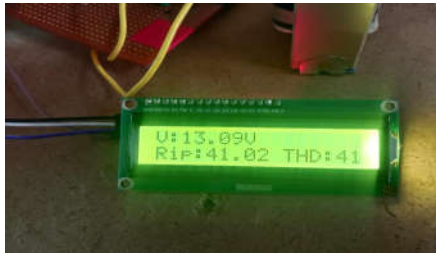
Fig 5.4.1 Output in THD Meter as observed Without filter
