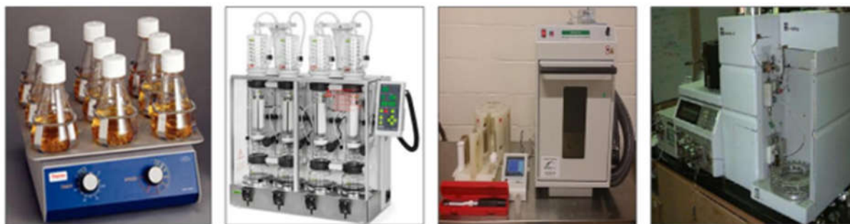
Figure. 1: Various techniques for extraction a) Solvent extraction; b) cold percolation; c) supercritical fluid extraction; and d) extraction with microwave assistance
