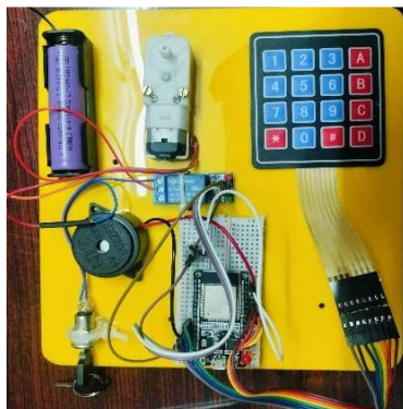
Fig-7 IOT based secured vehicle ignition control kit
