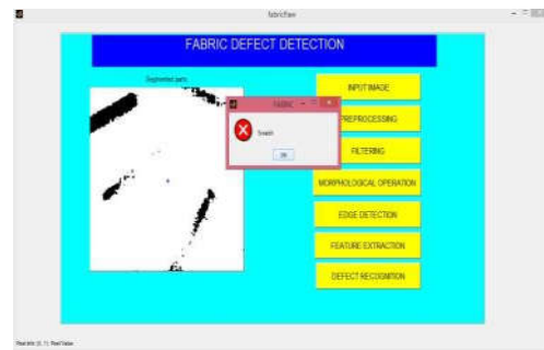
Fig 3. Dye spot detection
