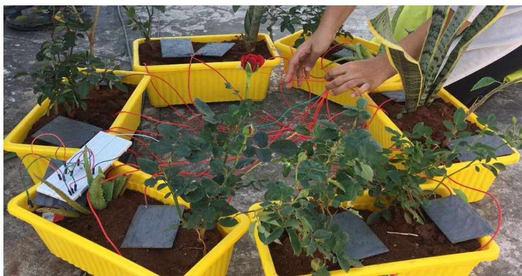
FIGURE. 4 Connecting plants in series to enhance the voltage
