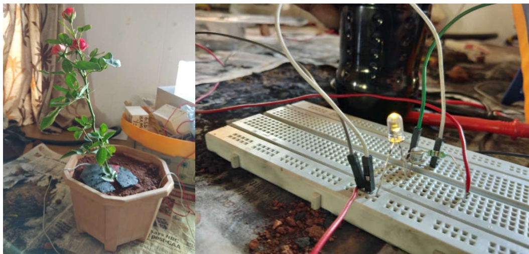
FIGURE. 3 Placing of electrodes inside the plant and connected to the circuit
