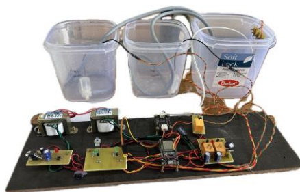
Fig. 2. Circuit connections of Aquaponic System
