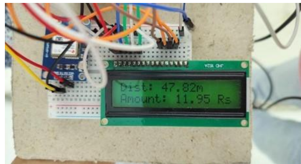
Fig.8. Distance and Fare readings after travelling for a certain distance at the endpoint (checkpoint)
