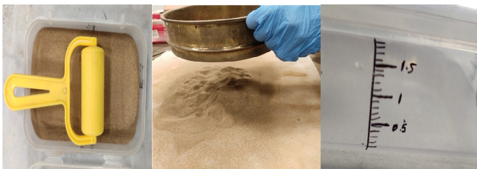
Figure 2: layering and sieving the soil sample using roller and sieve in plastic container with measurements
