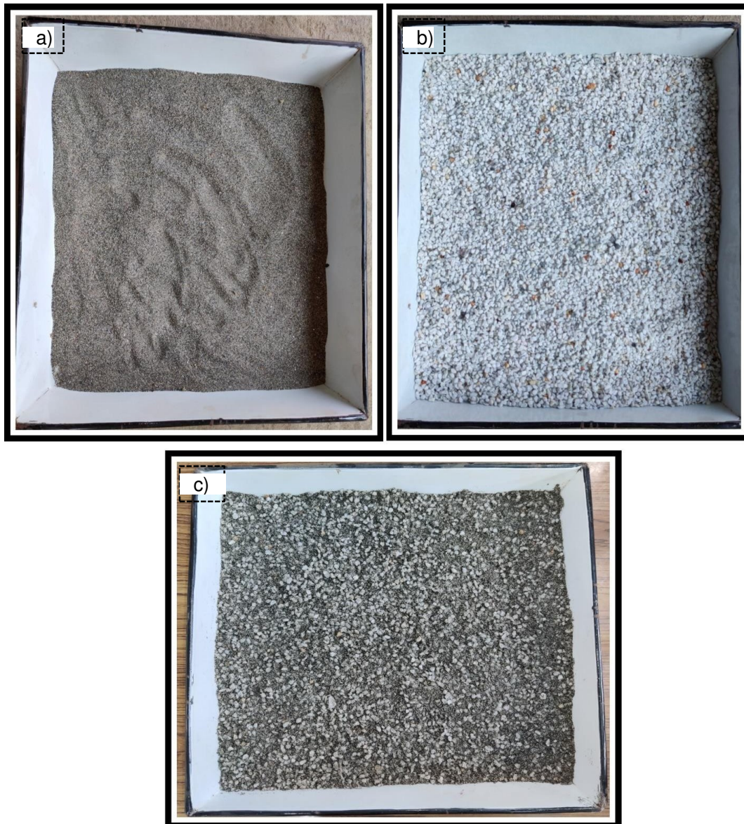
Figure 6. Cohesionless Sediments. a) Sand ( d_{50} ) = 0.27 mm, b) Gravel ( d_{50} ) = 3.52 mm, c) Sand Gravel mixture ( d_{50a} ) = 1.907 mm
