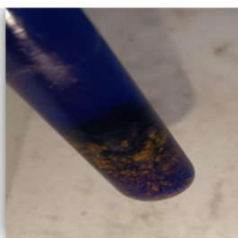
Figure 6: Laboratory Fehling's test for identifying furfural
