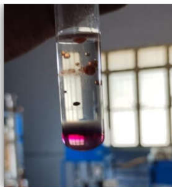
Figure 5: Laboratory Molisch's test for testing furfural
