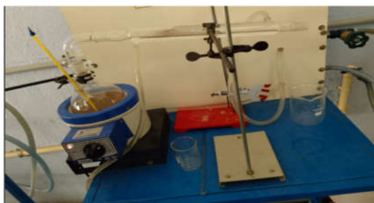
Figure 4: Distillation laboratory setup for furfuraldehyde production
