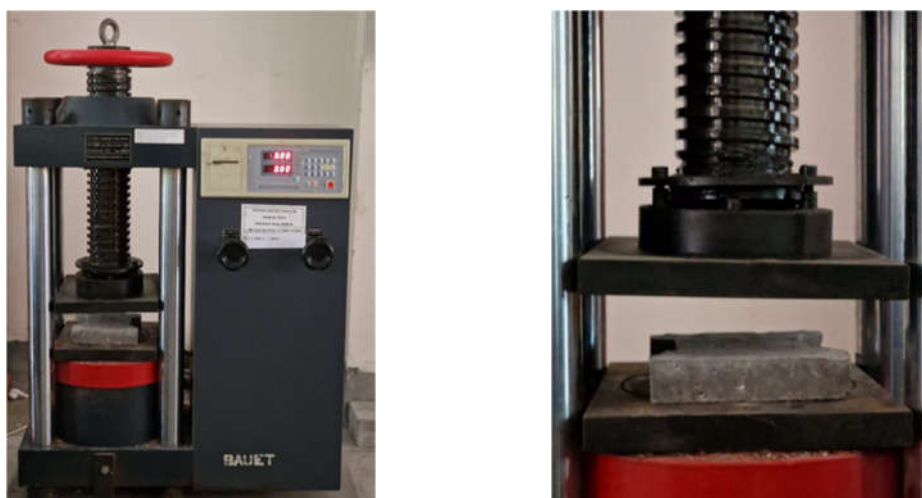
Figure 2: Compressive Strength Test of Pavement Concrete
