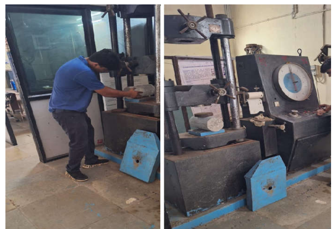
Image 8. Conducting Split tensile test on UTM
