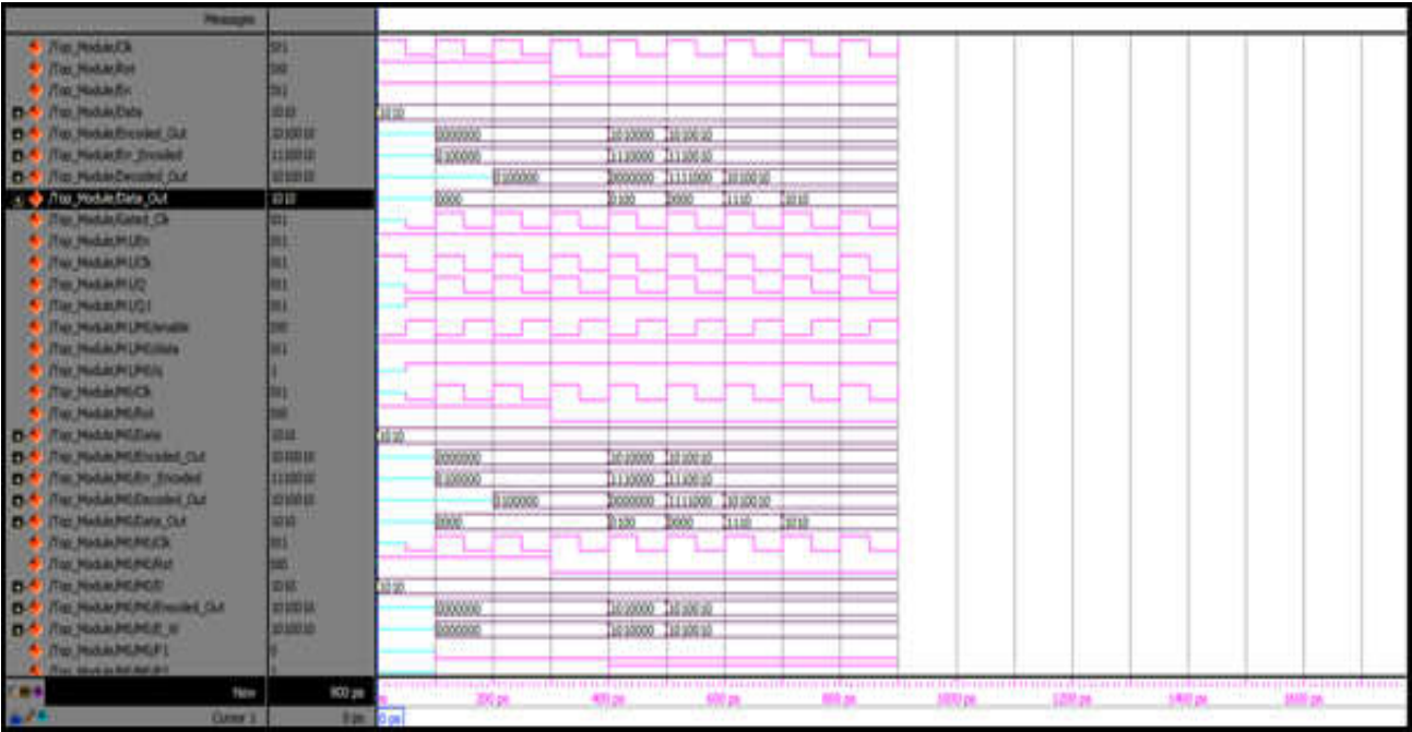
Clock gating based Encoder
