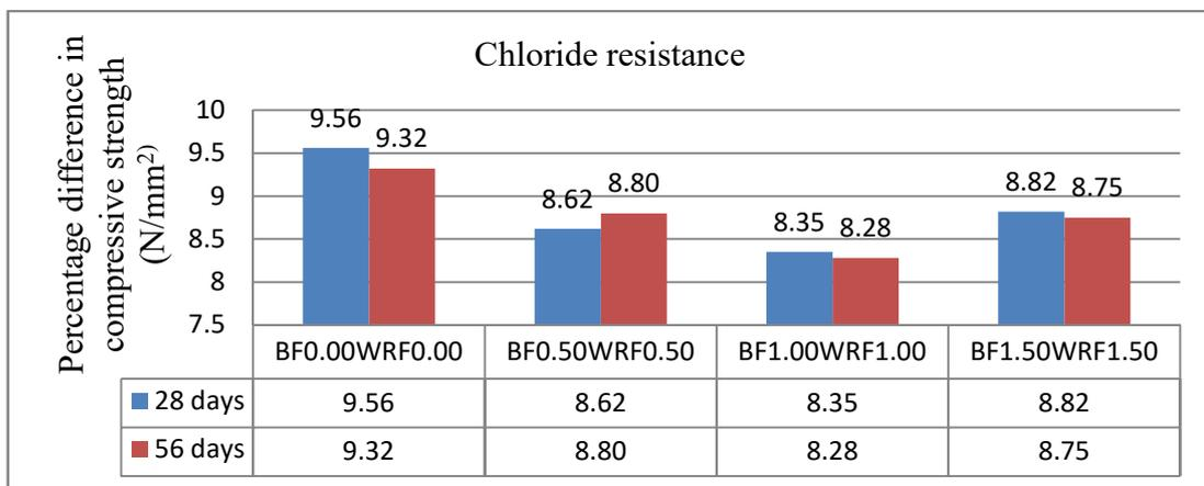
Fig 5.14 Effect of chloride on compressive strength of cubes
