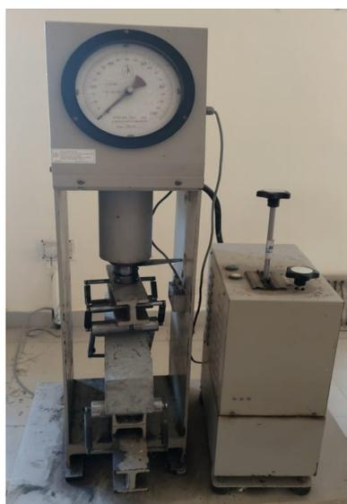
Fig.5.9 Flexural strength test set up
