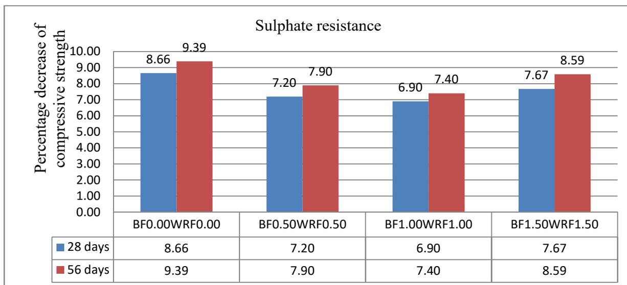
**Fig. 5.11 Percentage decrease of Compressive Strength (Sulphate Resistance)**
