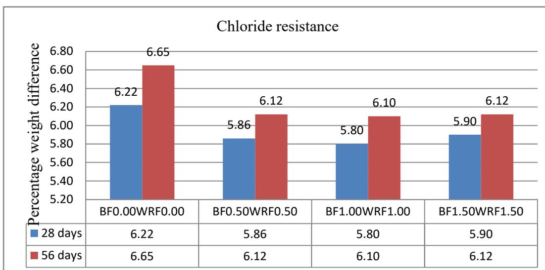
Fig 5.13 Effect of chloride on weight loss in cubes
