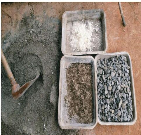
Fig. 5.1 Concrete mix preparation
