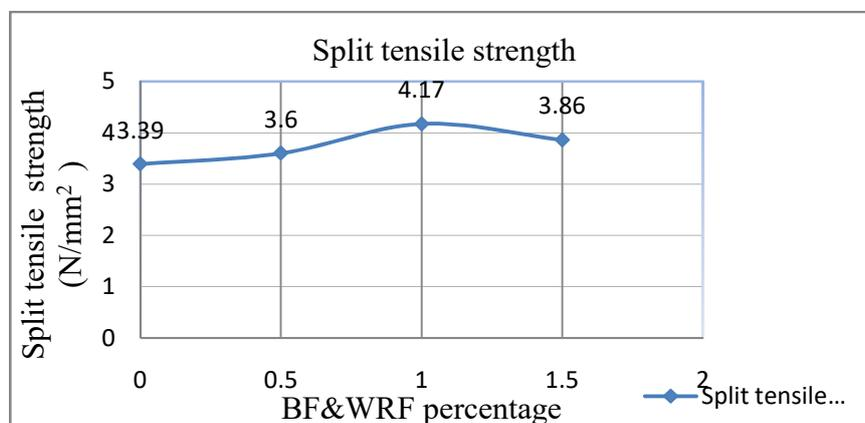
**Fig 5.6 Split Tensile strength vs BFWRF percentage**
