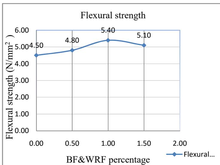
Fig.5.10 Flexural strength vs BF&WRF percentage
