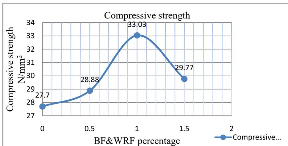
**Fig.5.4 Compressive strength vs BFWRF percentage**
