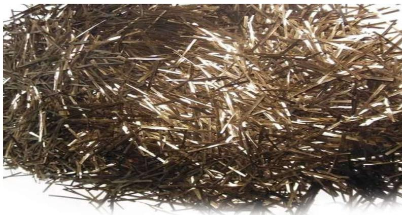
Fig.4.1 Basalt fiber
