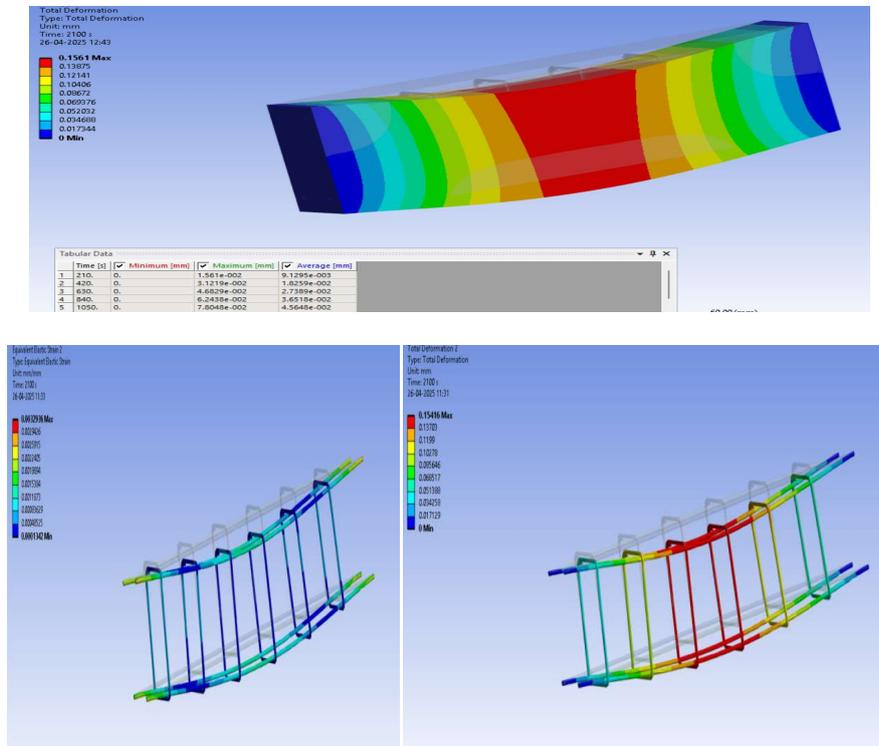
**Fig.6.8 Deformation diagram of beam with BFWRf1.00%**
