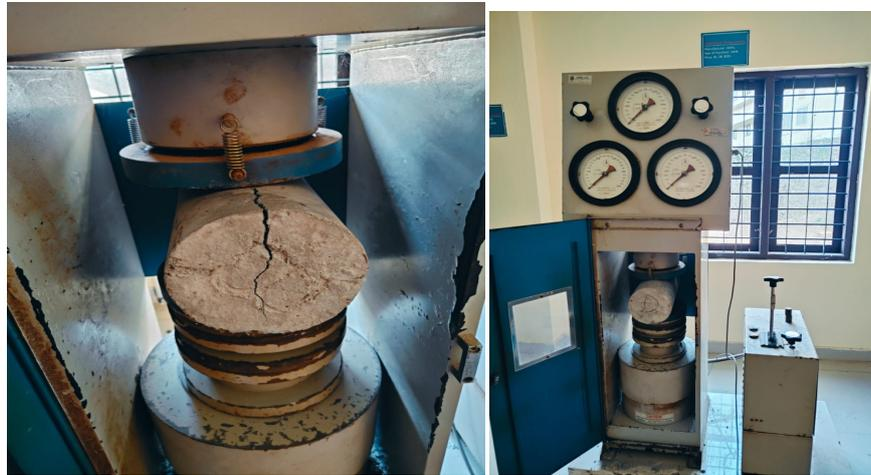
**Fig.5.5 Split tensile strength test set up**
