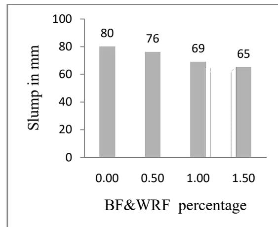
Fig. 5.2 Workability results of BFWRF mixes
