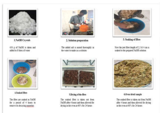
Fig No 2.3.2 NaOH Treatment Process
