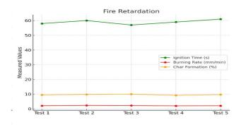
These findings support the ceiling board's good fire resistance, which includes a long ignition period, a sluggish spread of flames, and adequate material stability throughout combustion.
