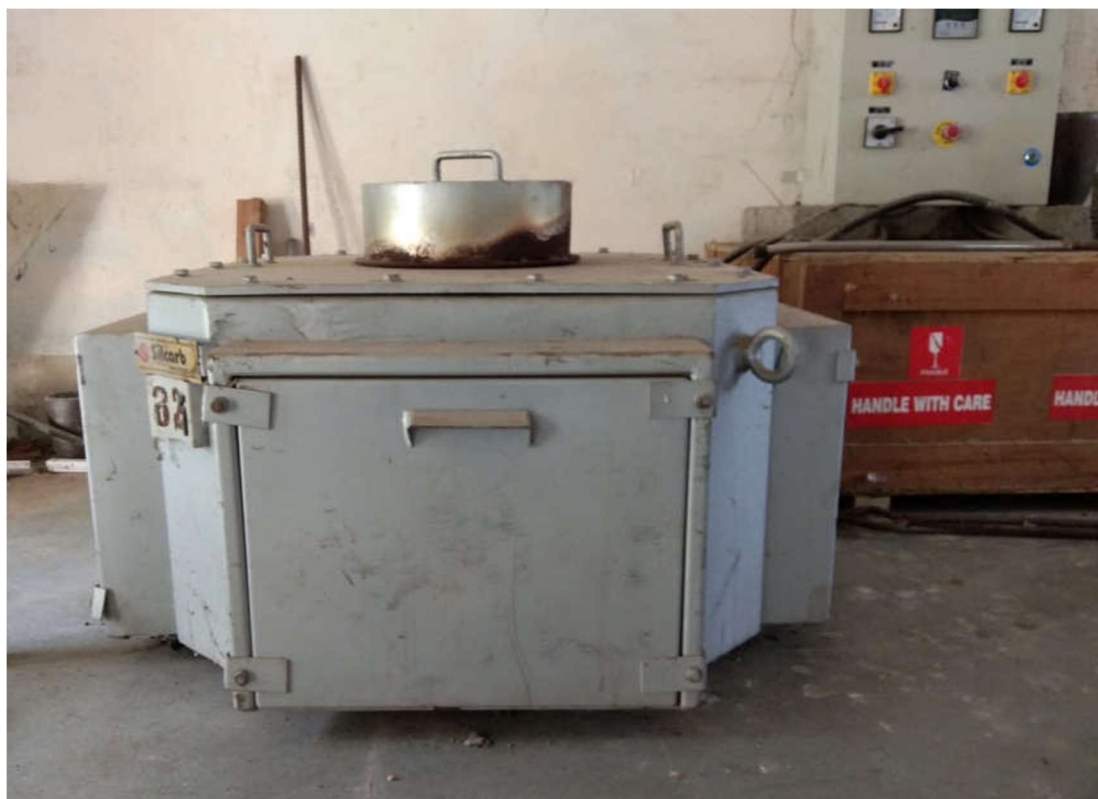
Fig.1 Electric resistance furnace with controll unit.
