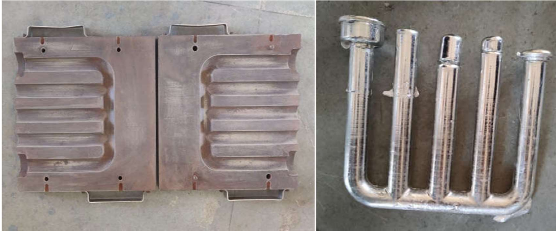
Fig.2 (a) Metallic Die (b) Casting after solidification
