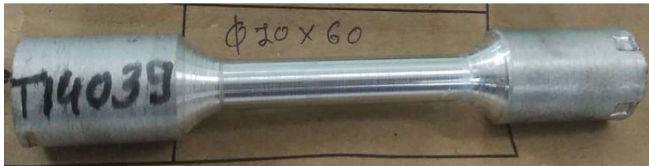
Fig.3 Size of Tensile specimen
