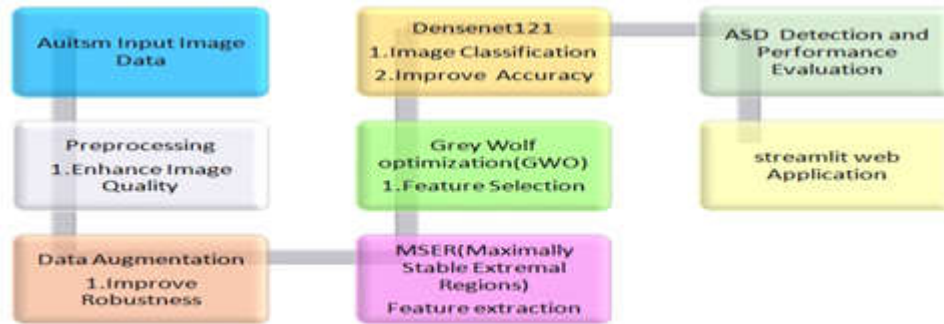
Figure .Proposed Block Diagram-GWO with Densenet121
